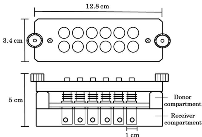
Fig. 1. Schematic representation of currently designed diffusion cell array system.
